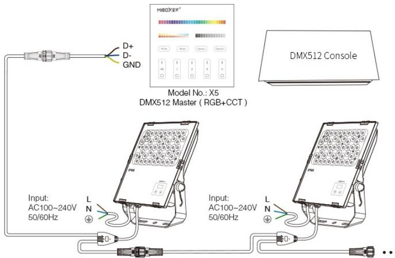
**Attention:** If more than 32 pcs DMX garden lights are connected or using the super long signal cable, you need DMX signal amplifier. Amplify signal cannot be over 5 times.
