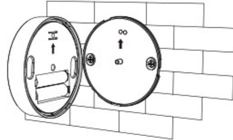
3. Press downward and rotate to the left to fix it.
