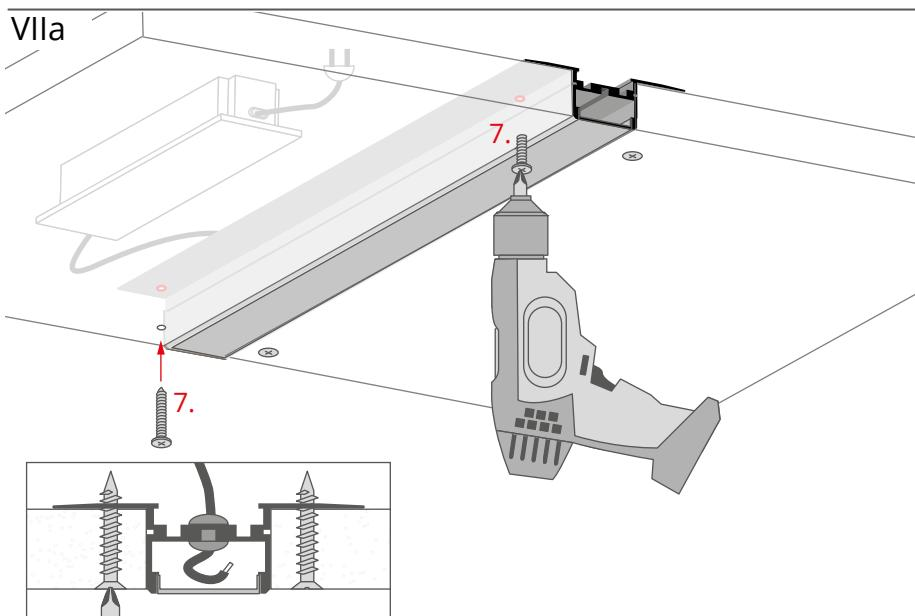
Insert the drywall screws (7) in the newly drilled holes and screw the second flange of the profile to the board.
