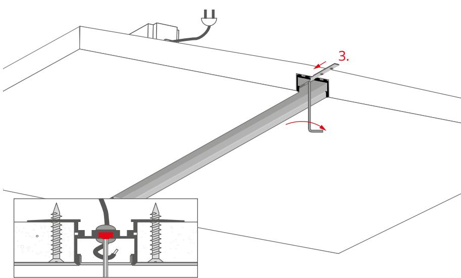
Insert the connector (3) into the channel inside the profile and tighten the locking bolts with an Allen key.
