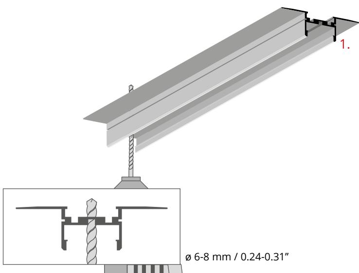
Drill a hole for the power cable in the GIZA-LL-UST (1) profile.
